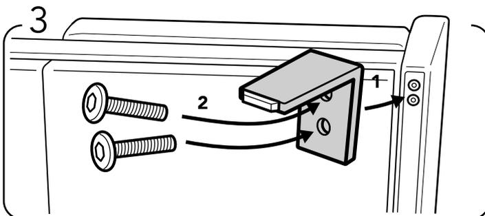
Mount the metal leg in place and screw the 2 (M6X25mm) bolts into the pre-drilled holes.
