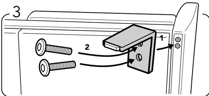
Mount the metal leg in place and screw the 2 (M6X25mm) bolts into the pre-drilled holes.
